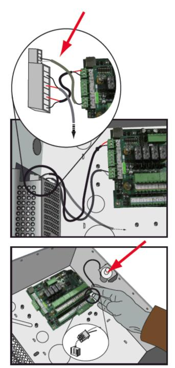
9. Power up the NetAXS-123 Controller Board and configure the system. Refer to the *NetAXS-123 Startup Guide* (800-05780) for instructions.
